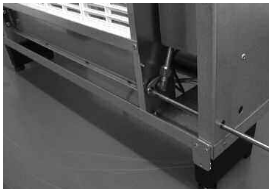
Fig. 11 Injector fixing bracket removal
