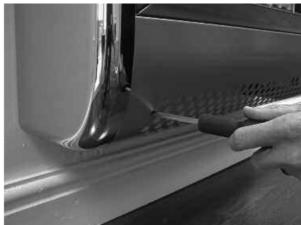
Fig. 4 Remove the Upper Outer Case Fixing Screws
