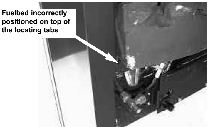
Fig. 26b - Shows incorrect location of fuelbed
